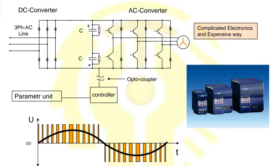
Inverter can produce Voltage with changed amplitude and frequency
