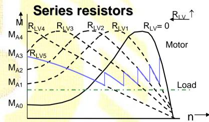
The starting torque is adjusted by matching the starting resistance to the rotor resistance.
