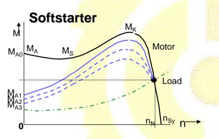
Soft starter reduces the starting torque
