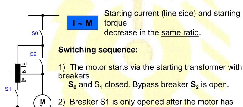
accelerated, and then bypass breaker  $S_2$  is closed.
